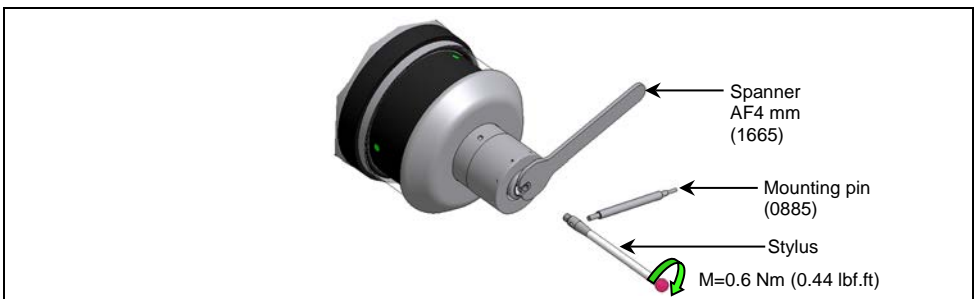
Fig. 11 Stylus change with measuring unit MY21.00
