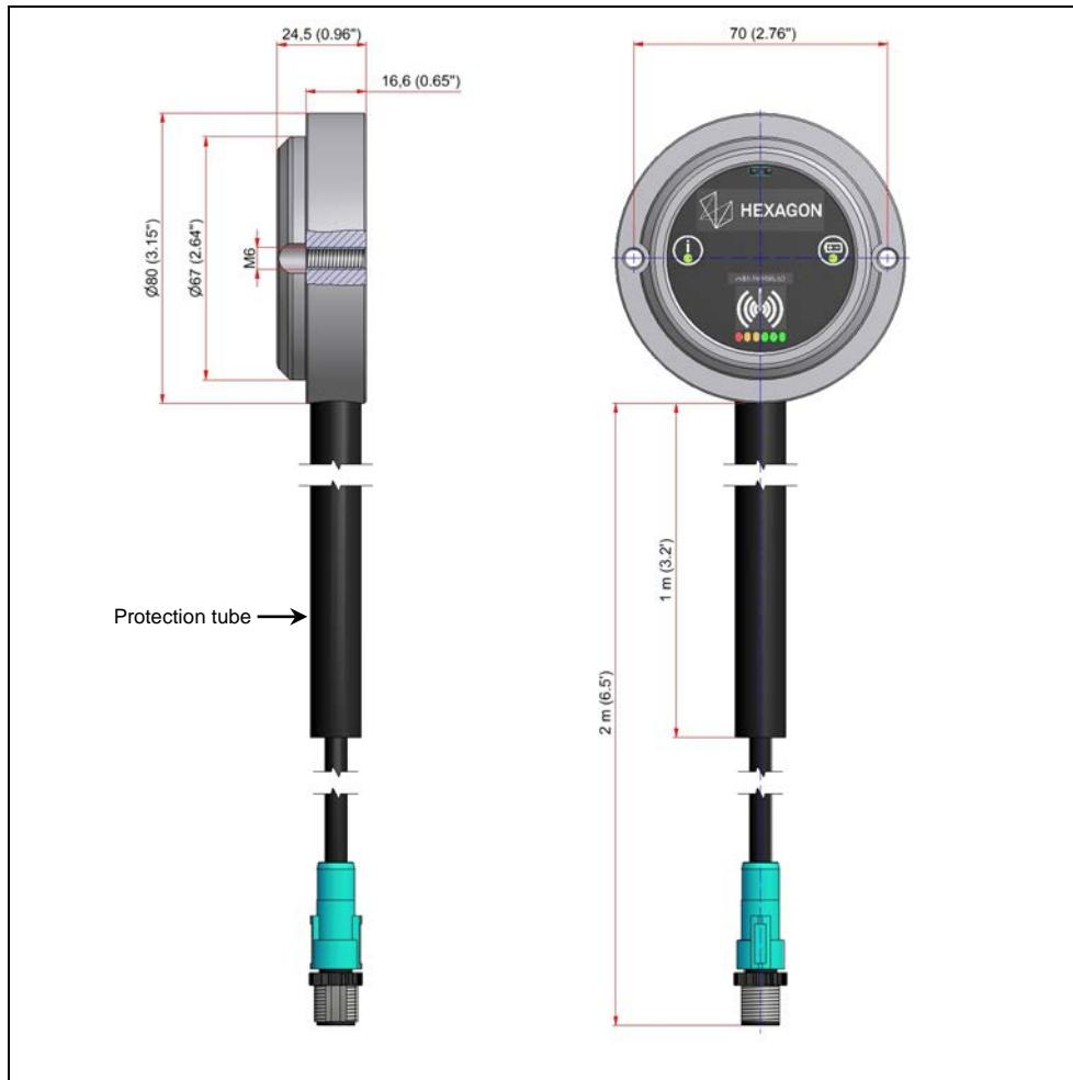
Fig. 5 Dimensions RWR95.50-A-PLUG-8 (cable outlet radial)
